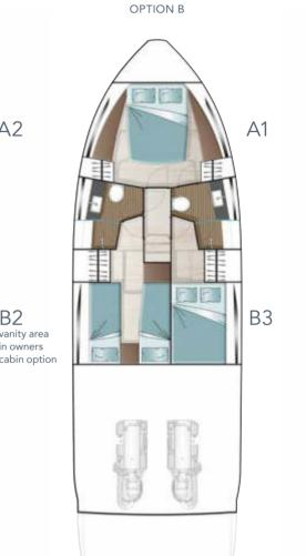
LOWER DECK aft cabin portside with twin bed and aft cabin starboard side with double bed
